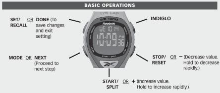
When setting, each button has a different function as indicated above. Display indicates when button changes function.
